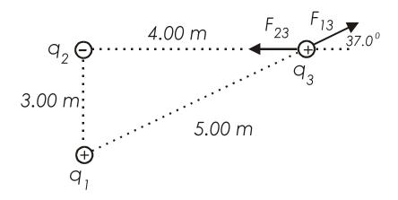
$q_3$  is attracted to  $q_2$  (they have opposite charges) and repulsed by  $q_1$  (they have the same charge). The two force vectors have been drawn and labeled,  $F_{23}$  and  $F_{13}$ .
